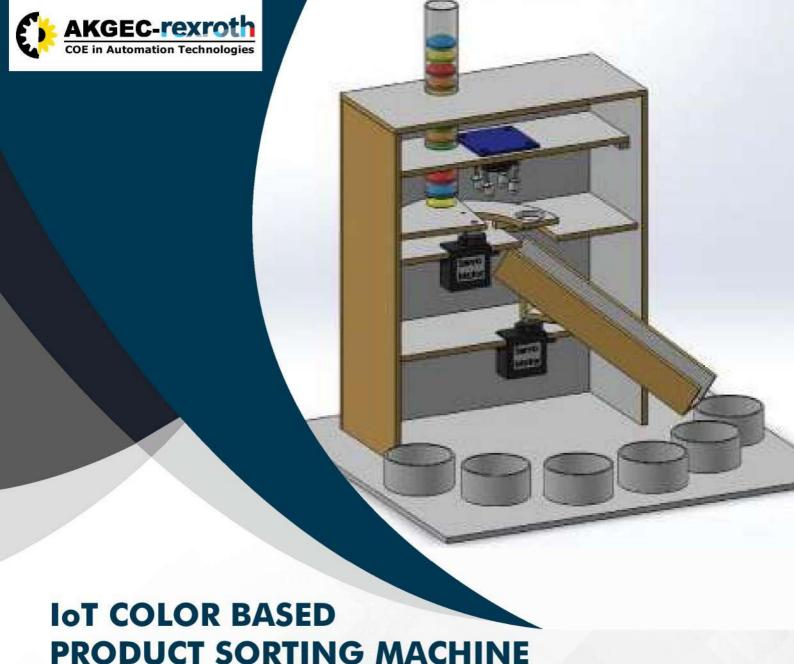
IoT based color sorting machine is a prototype of a machine that could sort objects based on their respective colors and send the data over the internet. It is a three-tier structure;
